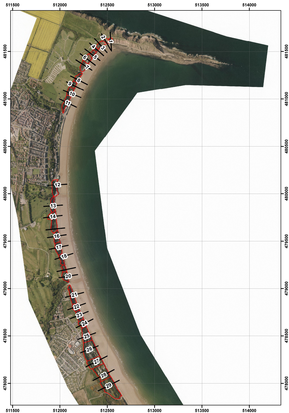
Figure 5. Location of transects used for coastal change analysis. Profiles 25 to 29 are reported here. Other profiles have been reported under the Filey town coastal slope study.
